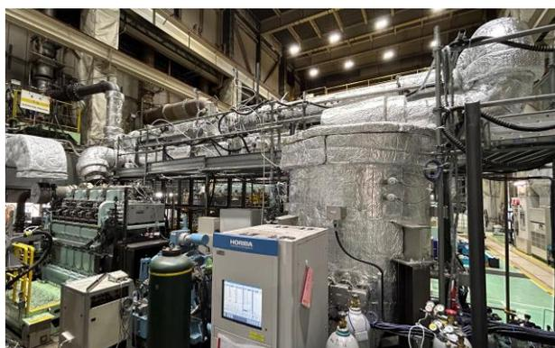
[Methane Oxidation Catalyst System Test Bench]
